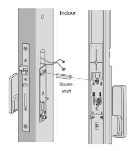
8. Tighten the 2 fixing screws.
