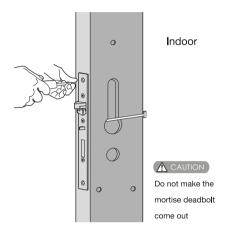
3. Fix 5 screw bolts on the front panel, place square shaft and pressure spring into the bore.
