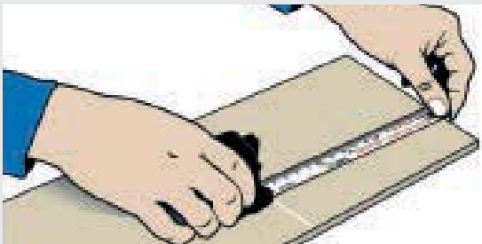
Transferring the measurement onto the workpiece
