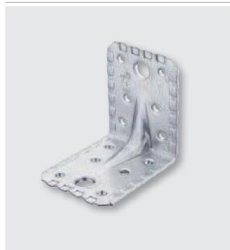
Symmetrical design around the pre-bending line, extremely high stability is achieved due the moulded ridge (reinforced rib) and folded edges; can bear higher loads than comparable angle brackets with thickness of 2.5 mm despite the narrow material thickness
