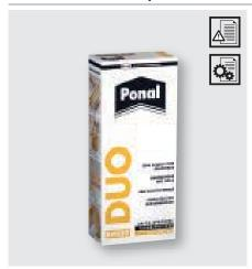
For the repair of construction elements made of wood and wooden materials for indoor and outdoor use with surface protection, open time approx. 15 minutes, can be sanded after 4 hrs., can be coloured with coloured paste Standard: Stress group D4 in accordance with DIN EN 204, and gap bridging in accordance with DIN EN 205
