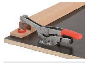
Characteristics: Horizontal toggle clamp with open arm, area of application: Clamp more flexibly and up to 5x faster, sensitive workpieces with a veneered or lacquered surface, for example, can be clamped without damage, adapts to workpieces with different thicknesses with approximately equal clamping force, without manually adjusting the pressure screw Version: extremely wide tightening range thanks to patented mechanism, clamping force regulation via adjusting screw in joint
