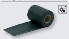
For sealing connection joints of windows/façades in outdoor areas vapour diffusion permeable, airtight, windproof and resistant to driving rain, waterproof, flexible and tear-resistant (sd value 3.7), self-adhesive on one side, pre-mounting on façades possible, additional mechanical fixing is not required when applied overhead, bitumen-compatible, UV resistant
