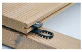
For invisible decking board fitting, for all decking boards with thickness of 20-26 mm and central groove with depth of 4 or 9 mm Tightening range: 5.5–11.5 mm, approx. 15 spacers are required for one m<sup>2</sup> Supplied with:
