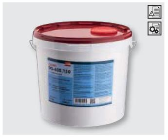
Single component D4 white glue, PVAc based Cosmo DS400.130 in compliance with DIN EN 204 (D4), open time approx. 12 minutes, press time approx. 22 minutes, one-sided application onto carrier material Processing temperature: from +8 °C
