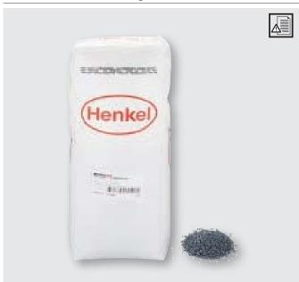
For edge gluing with feed rate from 15 m/min. Edge banding material: Veneer, melamine, polyester, HPL\*, PVC\*, ABS\*, PP\* \*up to thickness of approx. 2 mm
