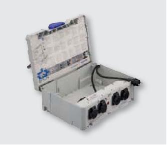
Stackable and connectable, also with systainer® Tool-Box 1, systainer® T-Loc and systainer® Classic line, IP44 dust proof and splash proof with 5 integrated 230 V sockets (4 x outside, 1 x inside) and extending 10 m cable with building site suitability (H07RN 3 x 1.5 mm²), 2x recess for cable guide, with control light, thermo switch for indoor use
