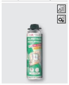
For insulating, assembling, bonding and filling, excellent shrinkage/post expansion stability, very low post-expansion, non-stick after approx. 8 minutes, can be cut after approx. 40 minutes, supports can be removed after approx. 120 minutes
