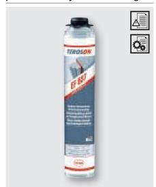
For insulating, assembling, bonding and filling (suitable for external thermal insulation composite systems), flexible single component expanding foam, gun version, with B1 quality for acoustic and thermal insulation of window connection joints, Colour: beige, flame retardant, Shearing strength: 4.0 N/cm² Standard: B1 in compliance
