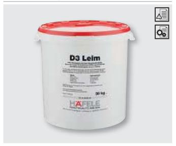
For bonding, for assembly bonding, for cabinet and joint bonding, PVAc based white glue Standard: In compliance with DIN EN 204 (D3), excellent water resistant properties, open time approx. 8 minutes, press time from 25 minutes
