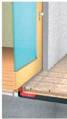
Consists of double-layer special foil with plastic art compound, rubber, bitumen, adhesive and sealing compound, seal against rising damp, leakage water, rain water and pressurised water
