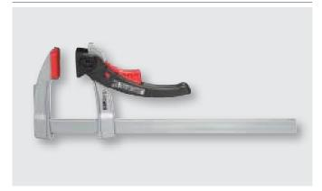
Gentle tightening due to swivelling pressure plate, lightweight and stable, clamping force up to 1,200 N Material: fixed and sliding jaw made of magnesium, ratchet made of glass fibre reinforced plastic Throat depth: 80 mm
