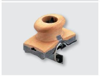
For sharp cutting and chamfering of plastic and veneer edges up to thickness of approx. 1 mm, can also be used for curves, stop continuously swivelling through 0 ° up to 45 °, forward and reverse use provided by double-bladed HSS knife
