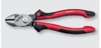
For cutting different materials such as cables, nails, screws, bolts, wire cable, spring wire or chains less force required, reduces the strain on the wrists, very convenient to use due to one handed operation, robust and durable, induction hardened cutters up to HRC 64
