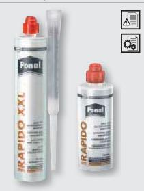
For fixing of door frames, steps and window sills, simple processing with cartridge gun, high stability during processing, assembly strips not required, can be cut after 4 minutes, loadable after 20 minutes, shrinkage/post expansion ±2 %, Colour: Green,
