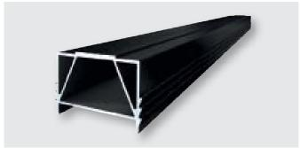
For quick and easy decking subconstruction, resistant against tannic acid, rotproof material, with support for underlaying Isopats (20 x 60 x 90 mm), max. distance of Isopats 1,100 mm (centre–centre of support points), total construction height (underlayment and Isopats): 57 mm Aluminium, black powder coated
