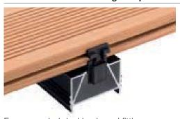
For concealed decking board fitting, for decking boards with central groove (width ≥ 4 mm; depth ≥ 9 mm), for use with substructures with aluminium rails and for laying decking boards with spacers for Isostep underlayment Glass-fibre reinforced polyamide
