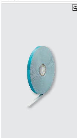
For mounting mirrors, for example, PVC window transoms and for mounting elements on tiles, smooth and rough surfaces, double-sided adhesive tape, dampens and compensates for vibrations, resistant to ageing, UV and softeners, final strength is reached after 24 hours Temperature range: -40 to +95 °C Length: 50 m
