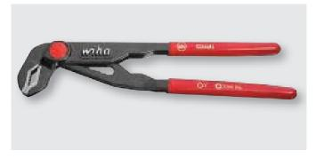
For gripping and holding tubes, profiles and hexagonal nuts, with push button adjustment for fast setting and locking mechanism, with extra narrow head for working in hard to reach places, optimum adaptation to object to be gripped by finely adjustable, through-bolt joint, robust and durable
