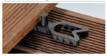
Made from recyclable plastic, Ensures the ventilation between decking boards and bearing beams as well as drying off wet dust, uniform decking pattern, approx. 15 spacers are required for one m2, bolt 7 mm
