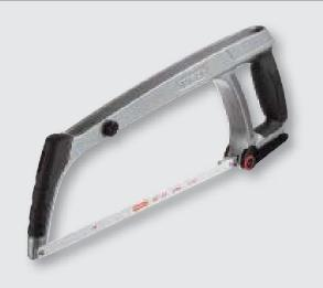
With sturdy metal frame, tension adjustment with clamping lever on the handle, easy blade change without tools, with support handle at the front, with non-slip handle, 127 mm cutting depth
