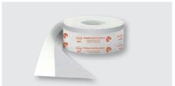
For sealing connection joints in indoor areas (warm side of the building), with façade, window and door elements, vapour diffusion retardant (sd value: Approx. 50 m), airtight and windproof, self-adhesive and can be plastered with Premium fleece (side dependent), adherent to wet blind frames, extremely tear-resistant, re-adjustable, additional mechanical fixing is not required when applied overhead
