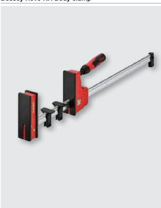
Very large parallel clamping surfaces with 3 removable protective caps to protect delicate surfaces, can be converted to spreading function without tools, high quality 2-component plastic handle with hexagon socket for comfortably reaching the clamping force (max. torque 17 Nm)
