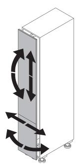
Just a standard PZ2 screwdriver and two setting screws at the top and bottom of the frame - simplify fine adjustment. Because turning the screws has an immediately visible effect. This makes adjustment quicker and easier - and also much more precise. And all it takes is a screwdriver!
