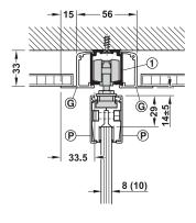
Ceiling installation with running track and  $2\ x$  clip panel for integration in suspended ceilings
