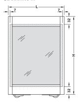
Panel size calculation Panel height: H – 64 mm Panel width: L – 14 mm
