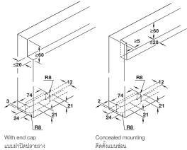
The lateral door overlap changes by ≥5 mm with concealed installation.
