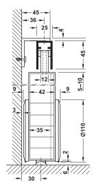
The wall distance of door is always the same, also with different door thicknesses. Please select different sizes of wall mounting brackets for extension of wall distance.
