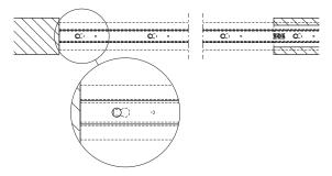
The running track is always clipped-in in direction of the locking point and secured with screws around the opening area.
