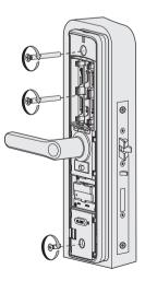
8. Install the batteries and the battery cover. Then install the striker assembly to finish the installation.
