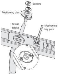
Reposition the sensor cable, so it is below arrow "△" sign on the positioning disc. Fasten the screws.
